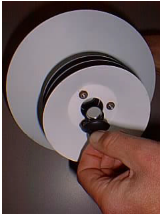
Small stacked plate screen designed for a single temperature logger.
